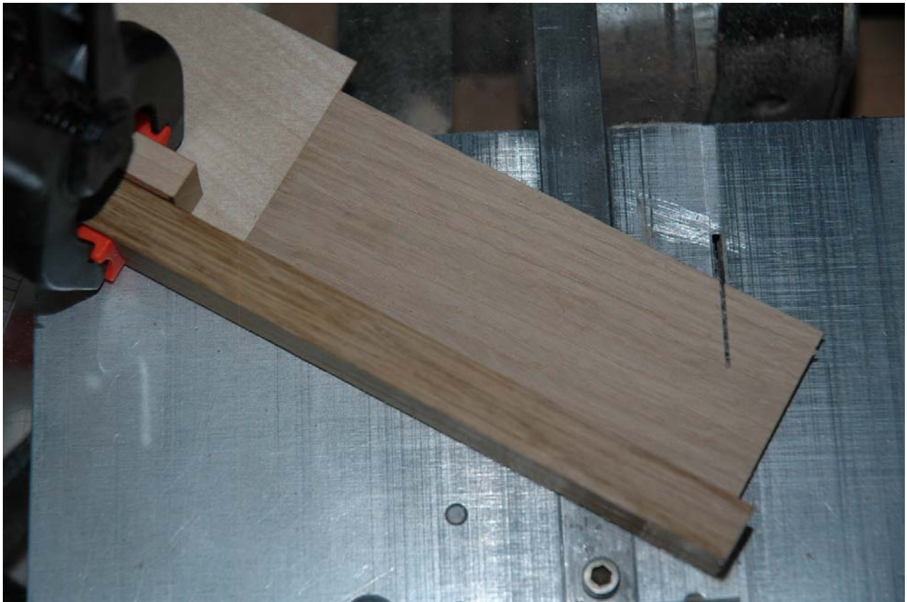
Figure 6 - Cutting the End of the Featherboard
