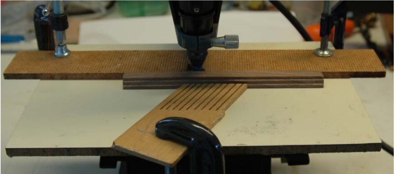
Figure 5 - Feather Board Setup for Moulding
