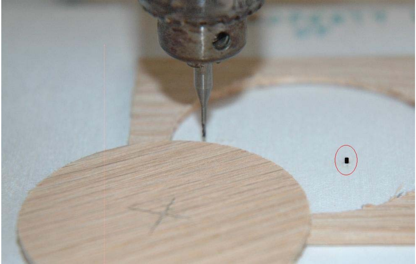
Figure 6 - Finished Circle Showing X Marking and Pin
