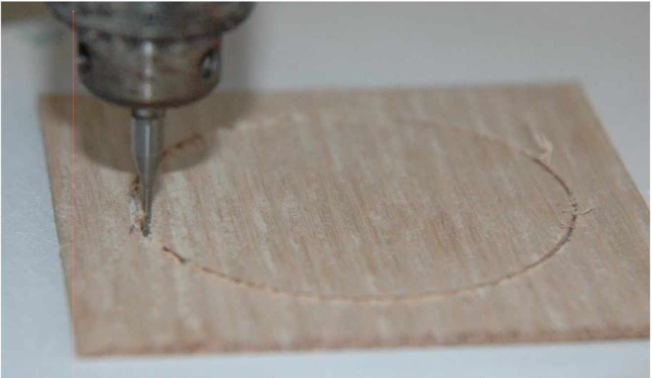
Figure 5 – Cutting a Perfect Circle with a Pin Routing Jig
